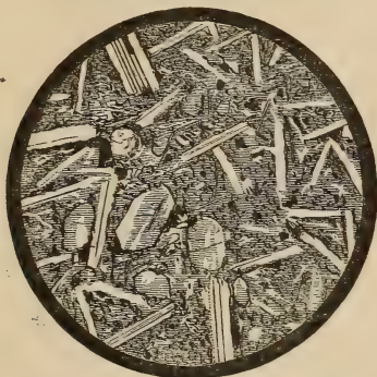
FIG. 11.—SEMI-CRYSTALLINE STRUCTURE. DOLERITE, CONSISTING OF A TRICLINIC FELSPAR, AUGITE, AND MAGNETITE IN A DEVITRIFIED GROUND-MASS (20 Diameters).
